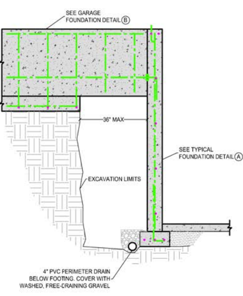
BASEMENT TO FOUNDATION WALL DETAIL
